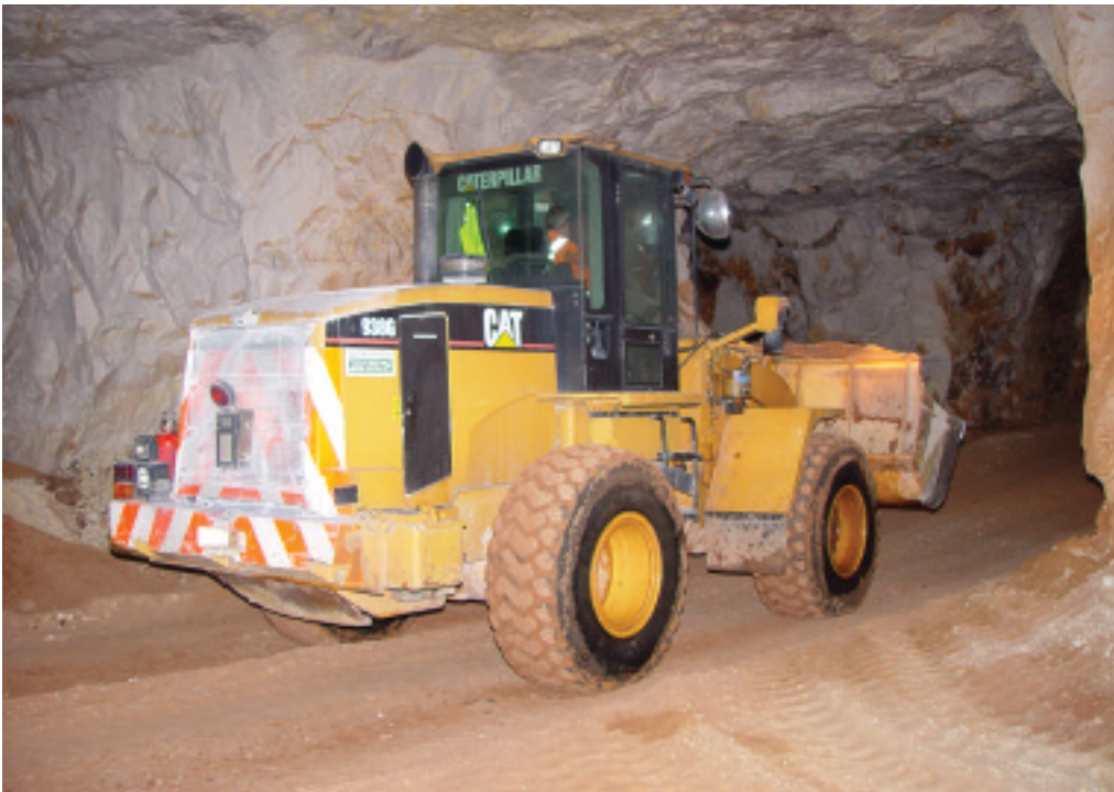
The Cat 938G loading shovel en route to the working face
