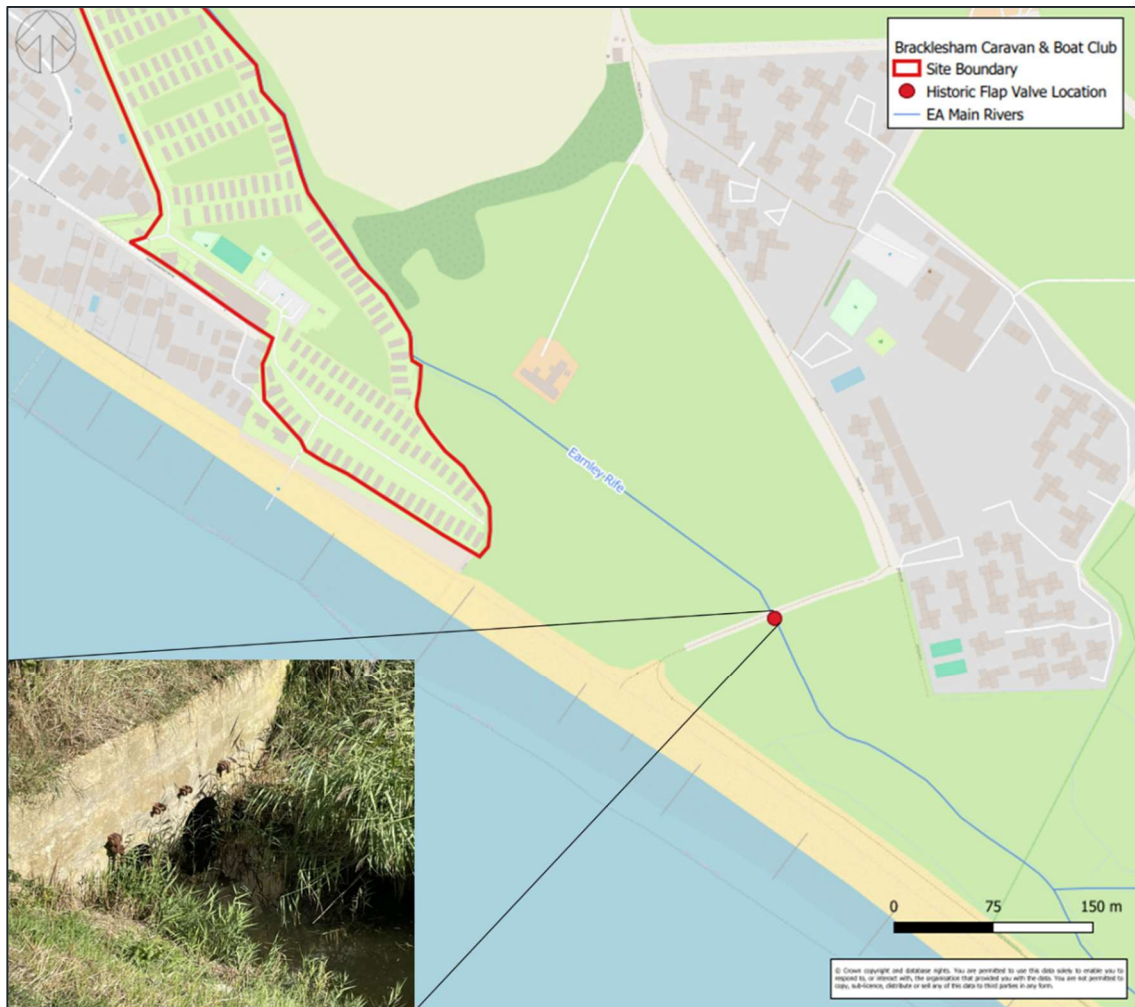
Figure 5-6 – Earnley Rife Culvert Location (note flap valve mountings on inset image)
